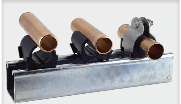
**CUSH-A-CLAMP** — Channel mounted clamping systems are ideal for multiple line runs, while absorbing shock and vibration, reducing unwanted noise, and preventing galvanic corrosion. Cush-A-Clamp fits any standard 41mm (1-5/8") wide channel.
